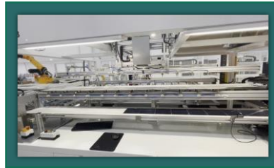
Inbuilt Stringer EL + VI Testing Facility
