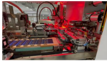
Stringer CCD checking Each Cells
