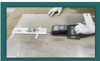
Backsheet to EVA & EVA to Glass Adhesive Test
